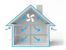
For homes with loft spaces, the PPS/L/H or PPS/L is installed in the loft and the discreet diffuser is installed in the hallway. For homes without loft spaces, the PPS/W/H is installed on the wall in a central hallway. Gently introducing tempered\* air into the house curing even stubborn condensation and issues.
