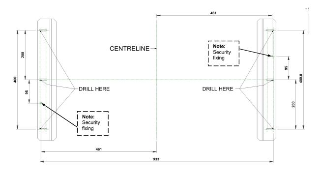
**Stage 1:** Drill the holes as shown above; make sure the holes you drill enable the brackets to be moved apart within the guide holes on the bracket.
