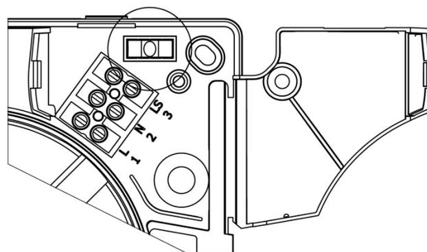
Open up the internal cover to access the spirit level bubble and terminals
