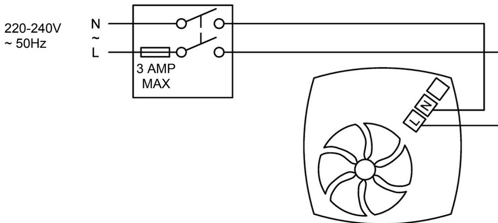
Fig.2: MONS100T/125T/150T/100HT/125HT/150HT (Timer /Humidistat disabled)
